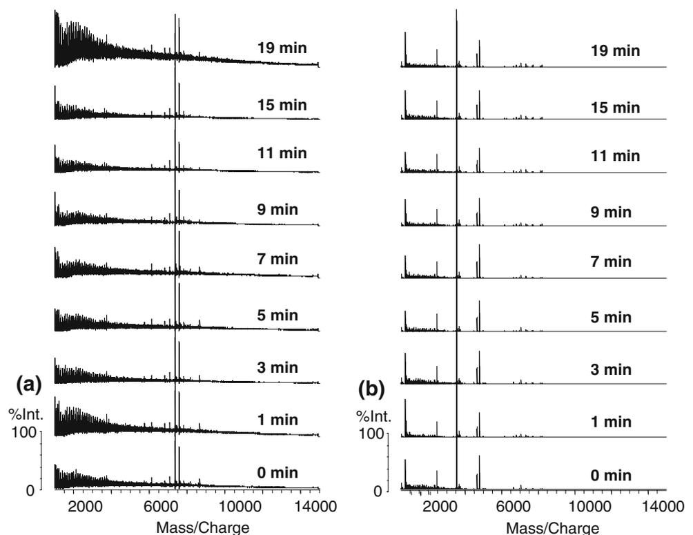
**Fig. 8** Repeatability of MALDI mass spectrometric analysis by the optimal sample preparation method developed in this study. **a** Six replicate MALDI mass spectra obtained from different spots of the same sample of *F. graminearum* strain 2765; **b** MALDI mass spectra derived from three different sample batches of *F. poae* strain 2786
