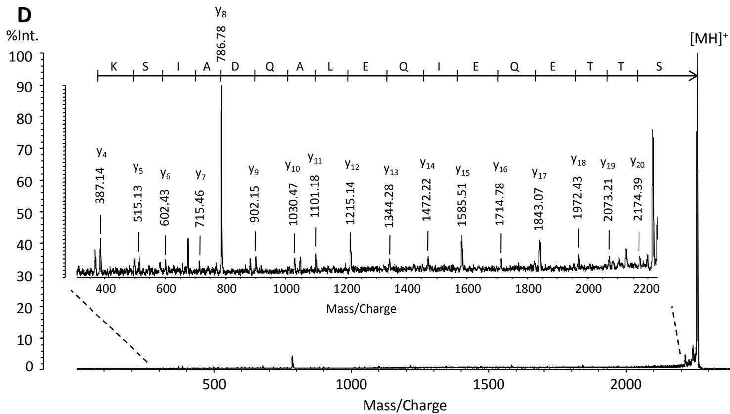
**Fig. 4 (D).** MALDI PSD (MS/MS) spectra obtained from the precursor ions at average  $m/z$  2261.3.
