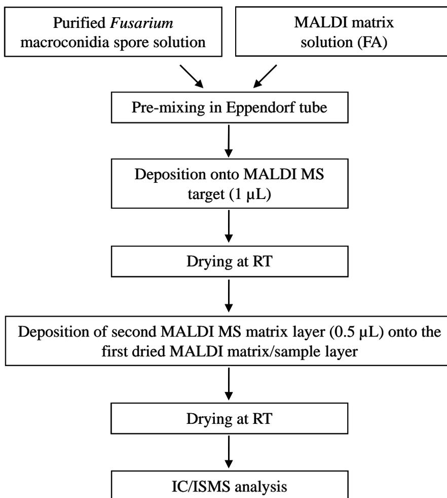
*Figure 3.* IC/ISMS sample preparation with two-layer volume technique for *Fusarium* macroconidia.
