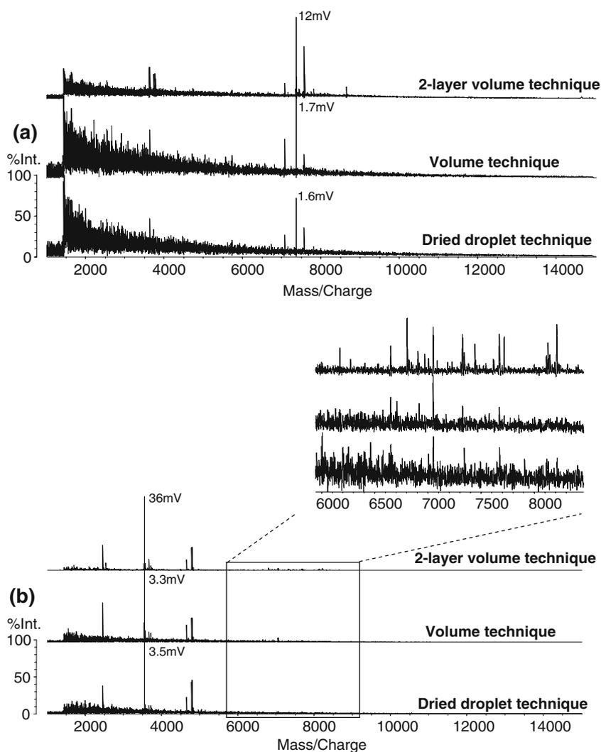
**Fig. 6** Comparison of MALDI mass spectra of intact *Fusarium* conidia pores using different matrix solution/conidia spore solution ratios applied with two-layer volume technique (**a**, left column) *F. poae* strain 2786 (light-colored) and (**b**, right column) *F. graminearum* strain 2765 (deep-colored). Matrix solution, 10 mg ferulic acid dissolved in 1 mL ACN/0.1% TFA (7/3, v/v); washing solvent system: ACN/0.5% FA (7/3, v/v); matrix solution/conidia spore solution mixing time, 3 min
