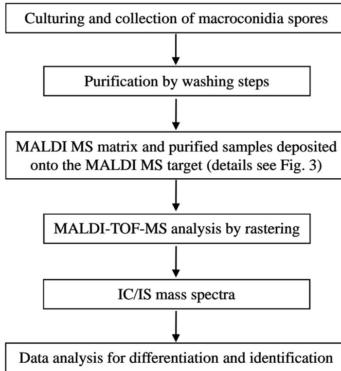
*Figure 2.* Strategy of intact cell/spore mass spectrometry (IC/ISMS) of *Fusarium* macroconidia.
