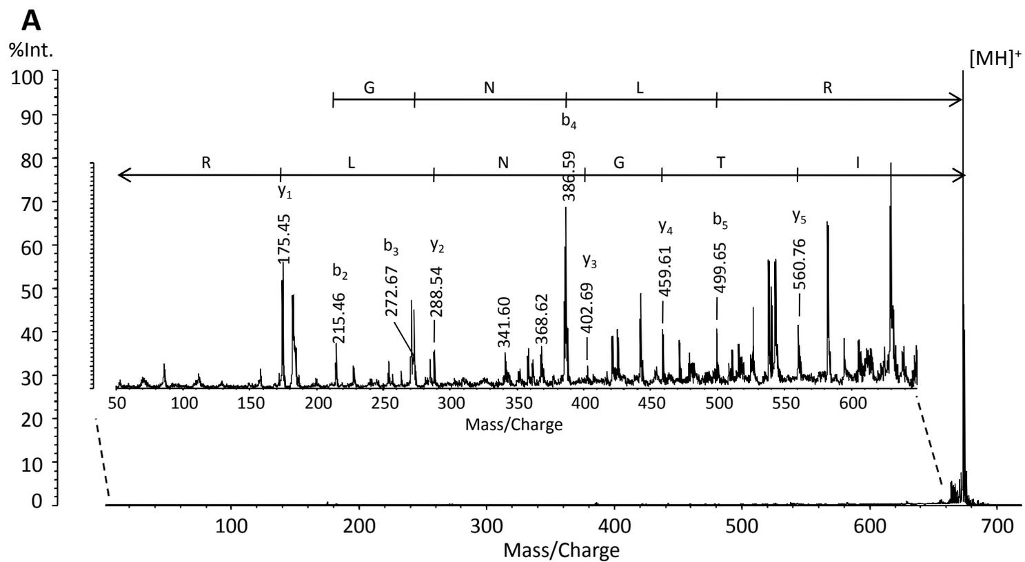
**Fig. 4 (A).** MALDI PSD (MS/MS) spectra obtained from the precursor ions at  $m/z$  673.7.
