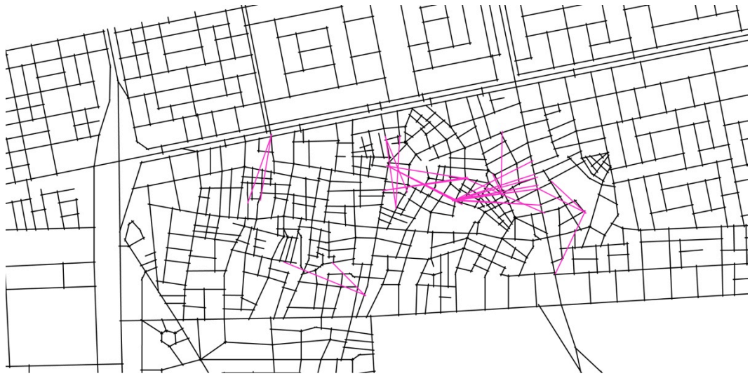
Figure 33: axial line map highlighting 1% of the most efficient new axial lines in scenario I
