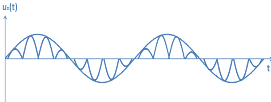
Figure 3-14: Synchronised signal u_D(t) .
