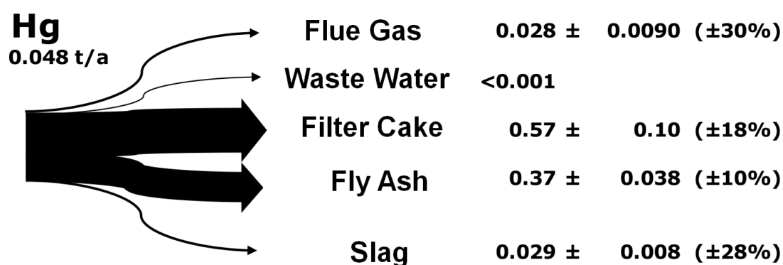
Figure 4.13 Transfer Coefficient for Hg in Spittelau incinerator (Rolland et al., 2011: 24)
