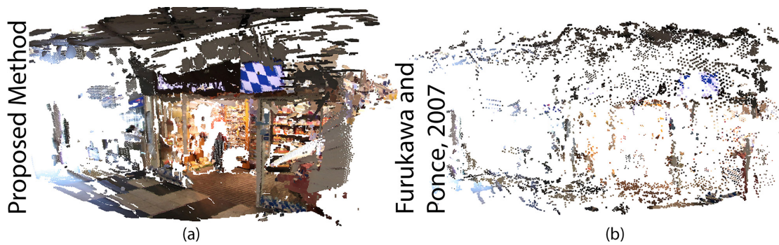
Figure 5.7: (a) Proposed semantic patch-based 3D reconstruction results compared to (b) conventional feature-based 3D reconstruction results [Furukawa and Ponce, 2007].
