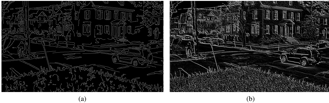
Figure 3.3: Edge features describing the structure of an image. (a) Canny edge detector using parameters \sigma = 3 , t_1 = 0.05 , t_2 = 0.2 , (b) Sobel filter without applying a threshold.
