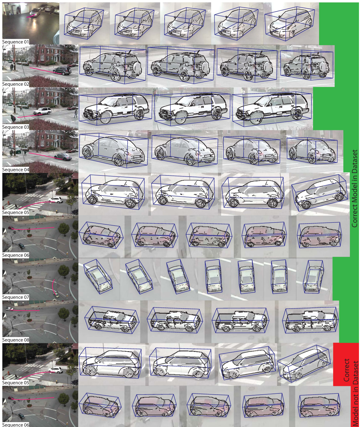
Figure 6.12: Qualitative results. One row describes one sequence where leftmost image shows first frame of it and the proposed optimized projected track. For rows 1-8, correct model is in dataset, for rows 9-10 it is not.
