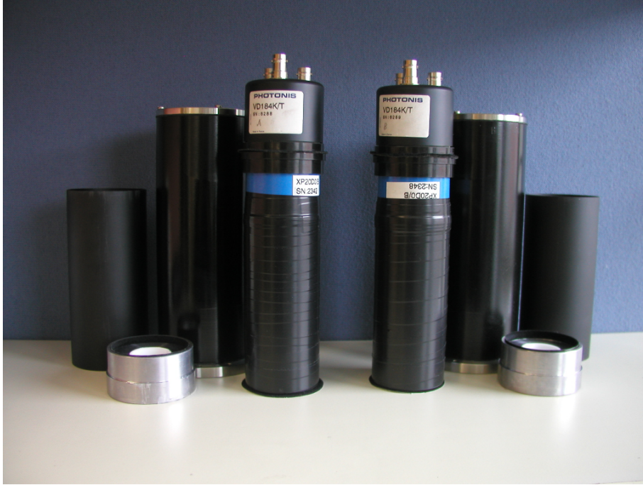
Figure 2.8: The picture shows all components included in both detectors. \mu -metal, lead ring with two layers of Teflon and the crystal in its centre, steel pipe with two flanges on top and bottom and the isolated PMT with the base mounted on its top (from outside to inside).
