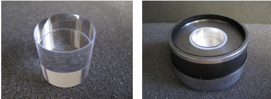
Figure 2.6: The LYSO crystal separately and surrounded by Teflon and the lead ring (the reflection foil cannot be seen in this picture). The felt stripe is glued onto the inner part of the lead ring to centre the PMT and to absorb the last light photons that might pass the outer light isolation. It furthermore provides additional electrical isolation which is necessary since the photo cathode is on high voltage.
