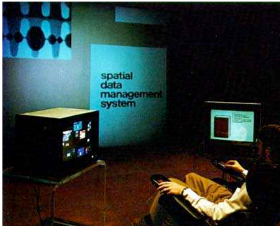
Figure 2.34: The Spatial Data Management System: A wall-size projection screen shows the detail view of a large data surface. A small display is used to provide a context view.
