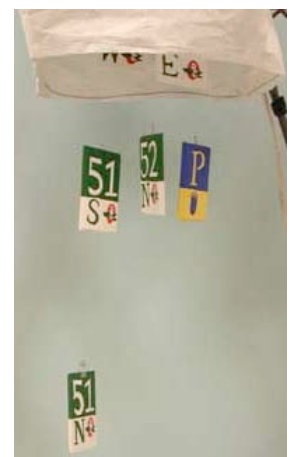
Figure 2.47: The Bus Mobile displays arrival time for busses. (Mankoff et al., 2003)
