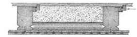
Figure 2.6: Composition of supporting wooden beams and floor and ceiling with fill for insulation.
