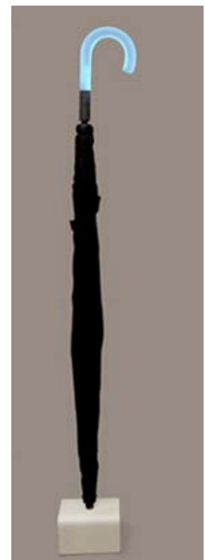
Figure 2.49: Forecast: an ambient display integrated into the handle of an umbrella to inform users about the weather forecast.
