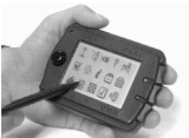
Figure 2.32: The PARCTAB Systems consists of small computers, called tabs. They feature constant connectivity and can be tracked through receivers.
