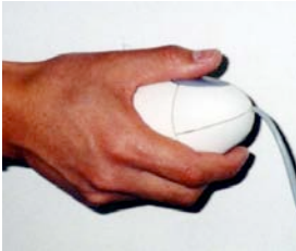
Figure 2.43: The GyroPoint device has a built-in gyroscope that supports operation in the air (Mackenzie & Jusoh, 2001).
