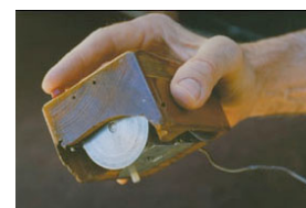
Figure 2.42: The first mouse developed by Douglas Engelbart in 1963.
