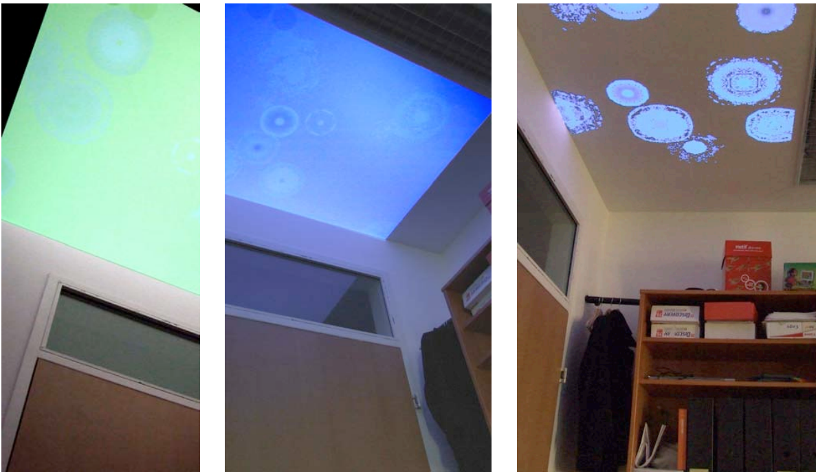
Figure 3.2: The first prototype for the weather forecast application showing warm (left) and cold temperature with rainfall (middle), and a revised version, where temperature was color-encoded into the graphical representation of the predicted weather condition (right).
