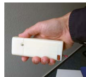
Figure 2.45: The Optical Tweezers system is a laser pointing device that uses three infrared beams to allow left and right button interaction in addition to cursor movement (Matveyev & Göbel, 2003).
