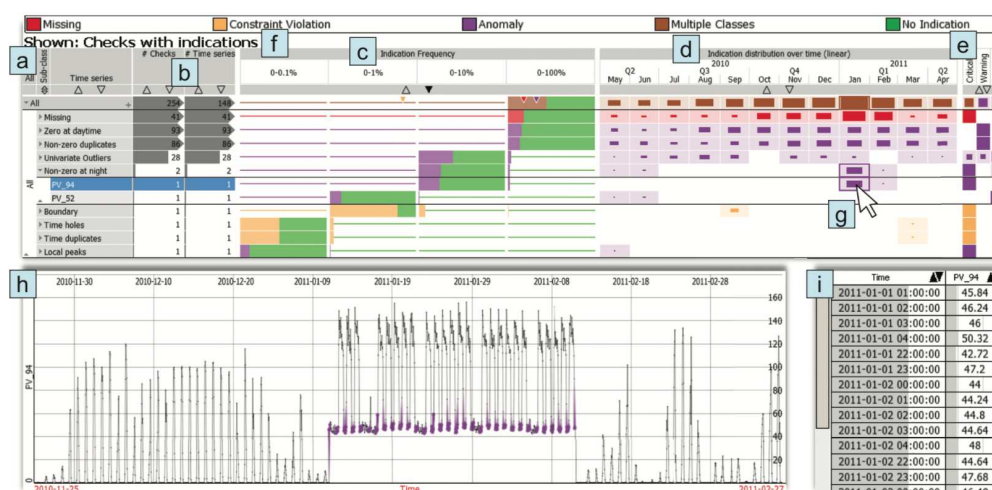
Figure 2.30: Visplause combines linked views: The central part is the DQ overview where analysts can explore the data by plausibility classes. Various time-oriented visualizations allow directed exploration of the data [ASMP17].
