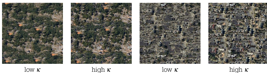
Figure 7.2: The images above demonstrate the impact of penalizing jumps within the similarity sets. The higher the value of \kappa , the more jumps are penalized. Low values of \kappa blur the image, but smooth out errors along the borders of the different tiles.
