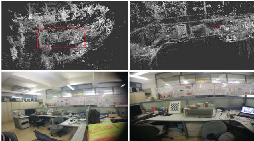
Figure 2.10: The final build depth map at the top with the corresponding real scene at the bottom [65].
