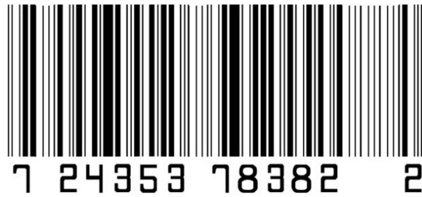
Figure 2.2: Example of a 1D marker [58], which can be used for AR orienting its renderings relative to the 1D marker position in the captured scene by the device camera.
