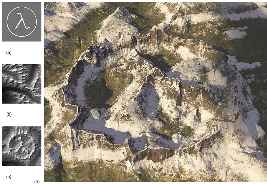
Figure 2.7: Synthesized terrain created using a data-driven method by Zhou et al. (a) Input user sketch. (b) Base elevation map. (c) Resulting synthesized elevation map. (d) Rendered result. [ZSTR07]
