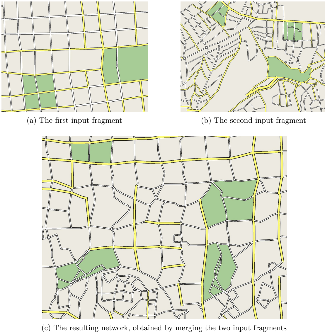
Figure 2.5: An example produced by the system presented by Aliaga et al.: Two street networks with different styles (a, b) get merged into a combined network (c). [AVB08]
