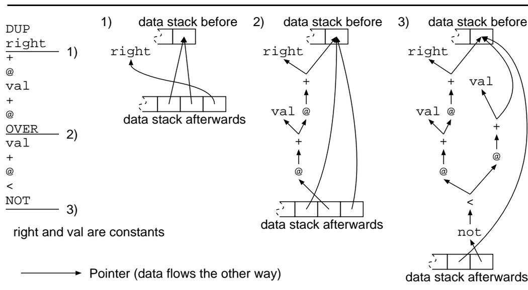
**Figure 3.1:** Building the data flow graph (three snapshots)
