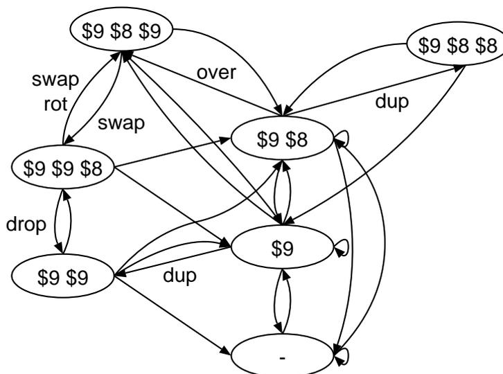
**Figure 2.18:** A cache organization where one duplication is allowed (`dup (x -- x x)` duplicates the top of stack, `over (x y -- x y x)` duplicates the second item, `swap (x y -- y x)` swaps the two top items, `rot (x y z -- y z x)` rotates the third item to the top, `drop (x -- )` pops the top item)
