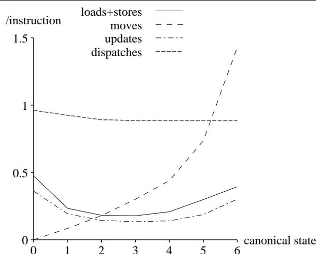
**Figure 2.27:** Static Stack Caching: Memory accesses, moves, stack pointer updates and instruction dispatches per (original) instruction of organizations with 6 registers for varying canonical states
