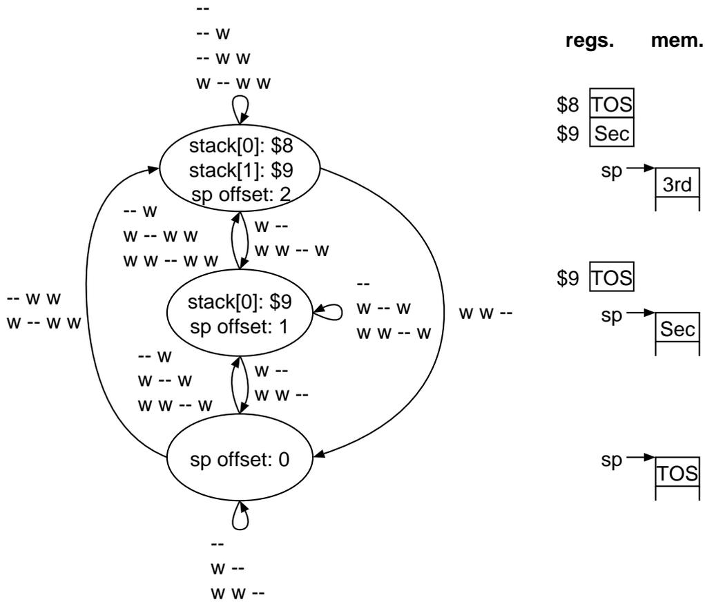
**Figure 2.14:** A simple cache state machine. Transitions are marked with stack effects; all instructions with the same stack effect perform the same transitions. The three states of the stack cache are also shown in a style similar to earlier figures.
