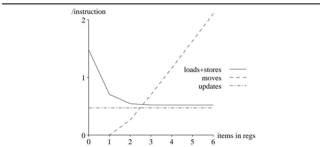
**Figure 2.23:** Keeping a constant number of items in registers: Memory accesses, moves, and stack pointer updates per instruction vs. number of items kept in registers
