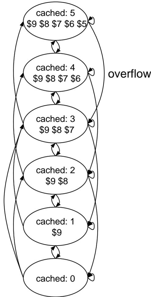
**Figure 2.16:** Overflow transition in a minimal organization (the top-of-stack is rightmost, \$9 contains the deepest cached item)
