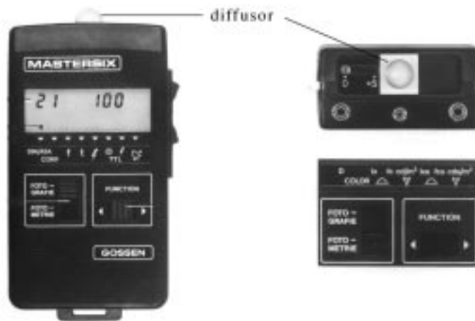
Figure 7.2: Incident and reflected light meter
