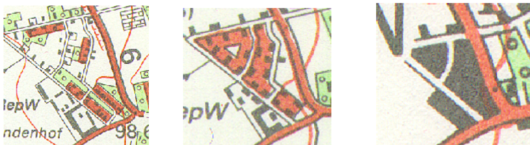
Fig. 6.1: Map clips at different levels of detail shown at same nominal scale
