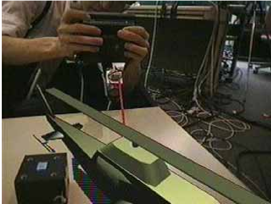
Figure 19. TransVision – By pushing the object selector button a beam is emitted perpendicular to the surface of the hand-held display device. The first object hit by the beam is selected for further manipulation.
