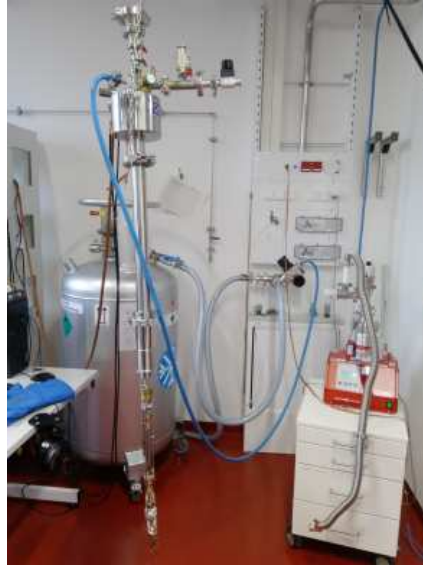
Figure 3.10: HelioxVL refrigerator used for the reported measurements.
