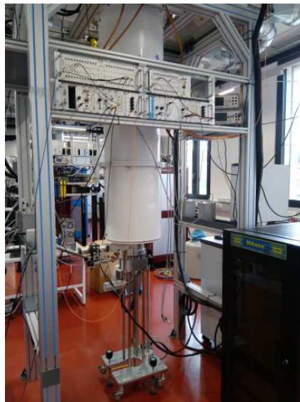
Figure 3.11: Blue-fors dilution refrigerator used for the reported measurements
