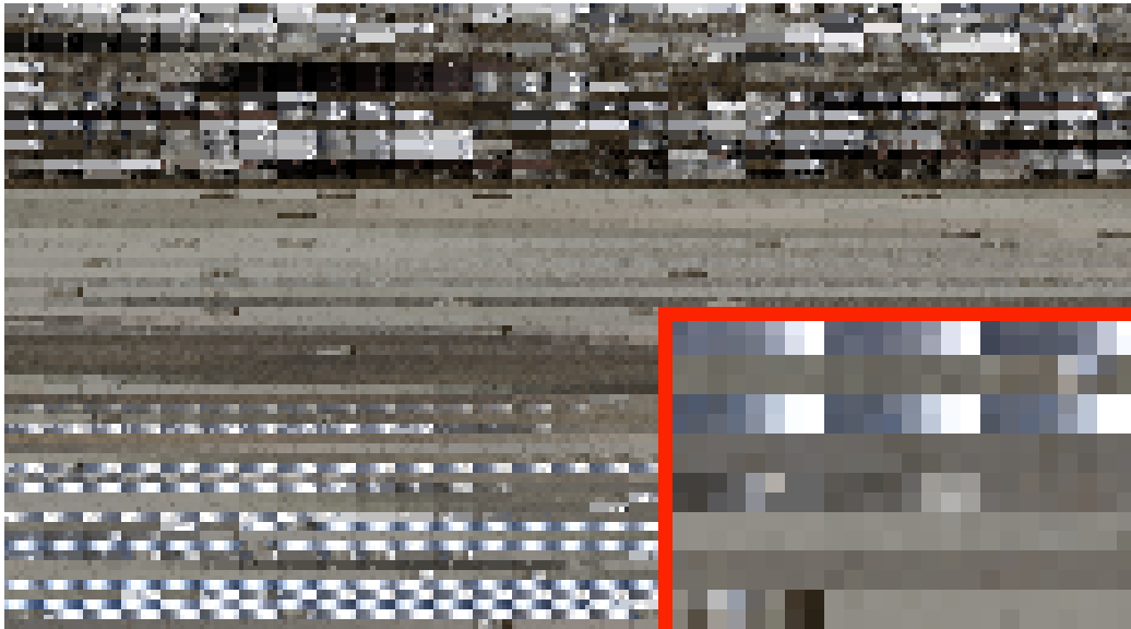
Figure 5.11: A 232x128 pixel (29x64 points) part of the packed texture for the impostor in figure 5.13. For each point, there is an 8x2 block in this packed texture. Note the bright blocks from the specular highlight. The inlay in the lower right corner is a zoomed 24x16 pixel part of the texture, showing the blocks for 24 points.
