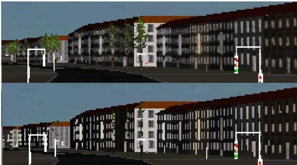
Figure 5.15: One frame of a city walkthrough. Note the correct filtering of the impostor (top) compared to geometry (bottom).
