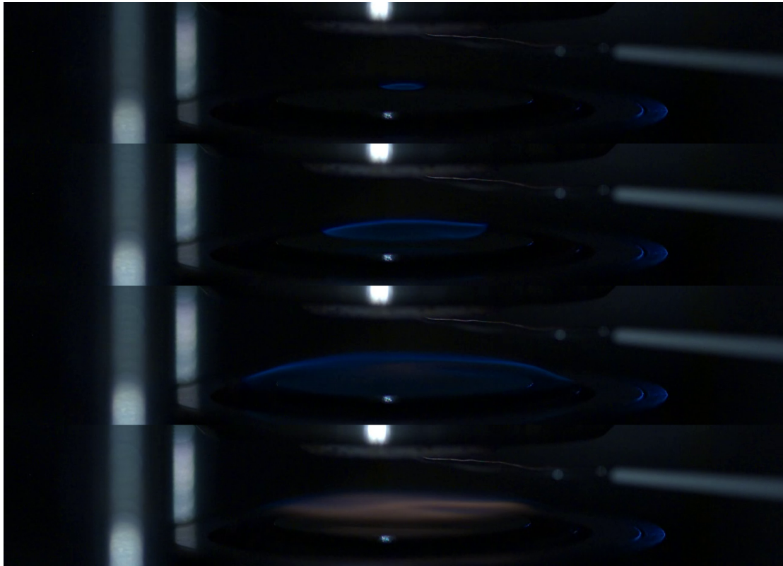
Figure 14: High speed image of an autoignition event with heptane with an oxidizer strain rate a_2 = 150 \text{ s}^{-1} and pure air as an oxidizer
