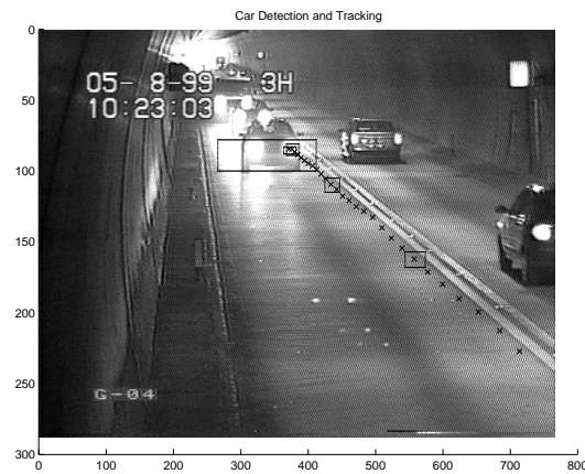
Figure 2.1: A typical frame of a tunnel scene video. The right car light of the visible car is pursued through the images. Each position is shown by a cross. Positions form together the trajectory.
