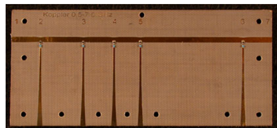
Fig. 3.35 - Standing Wave Probe with Resistors
