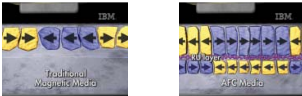
Figure 1.2: In traditional longitudinal magnetic recording media ferromagnetic grains represent one bit as shown in the left image. The demagnetizing field that occurs at the transition between bits can be reduced by antiferromagnetically -coupled (AFC) media as shown in the right image [5]. The opposing magnetic orientations make the entire multilayer structure appear much thinner than it actually is.
