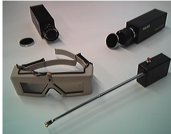
Figure 6.4: The tracking system equipment
