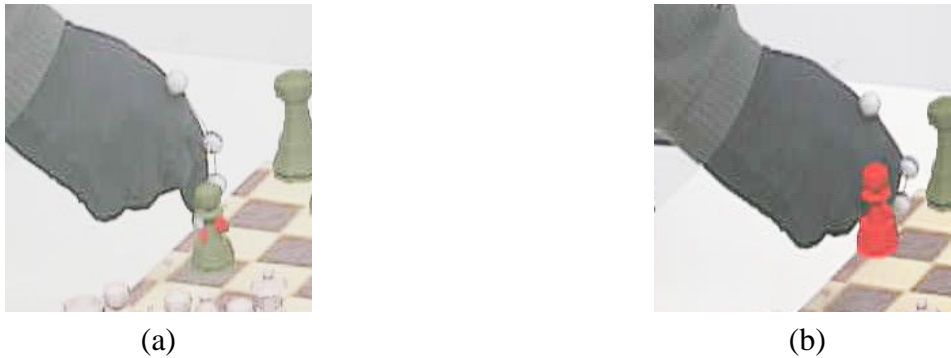
Figure 6.16: Manipulation of virtual objects by grab and release gestures: Natural interaction is possible using the finger tracker described in this section together with augmented reality displays. In this image, a user plays chess against the computer by moving virtual chess men with his finger on a real board.
