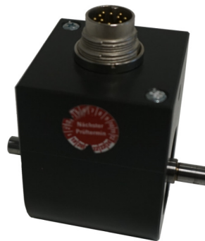
Figure 3.1: Rotary torque sensor used in the teach-in tool.
