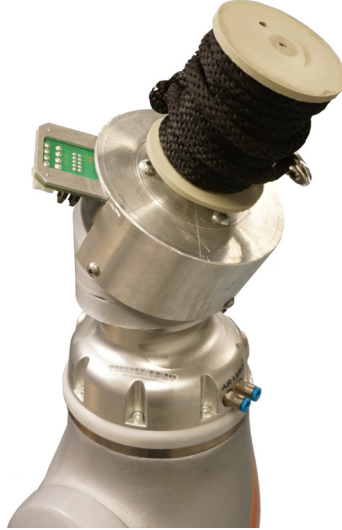
Figure 5.9: Spool and motor and the robot tilted around the y -axis, see also Figure 2.2.
