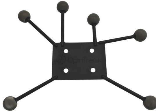
Figure 3.2: Marker body with infrared markers. This body is mounted on the teach-in tool for tracking the pose.
