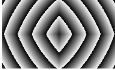
Figure 3.22: Eccentricity transform of a rectangle. (Gray values are distances modulo a constant.)
