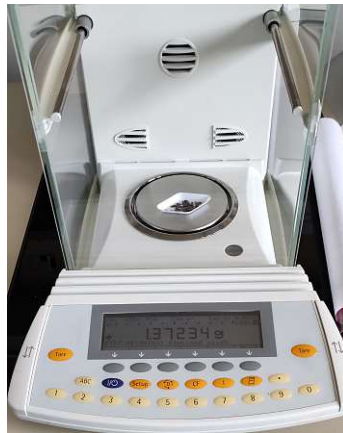
Figure 23: High precision scale for weighing the of sample components.
