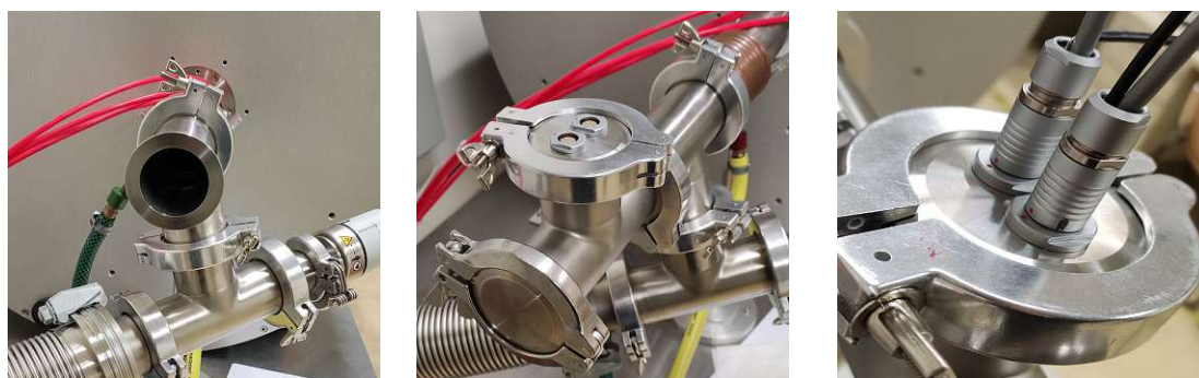
Figure 15: Installation of the sample holder. Tube system ready for insertion of the sample holder (left). Installed and fixed sample holder (middle). Connected wires (right).
