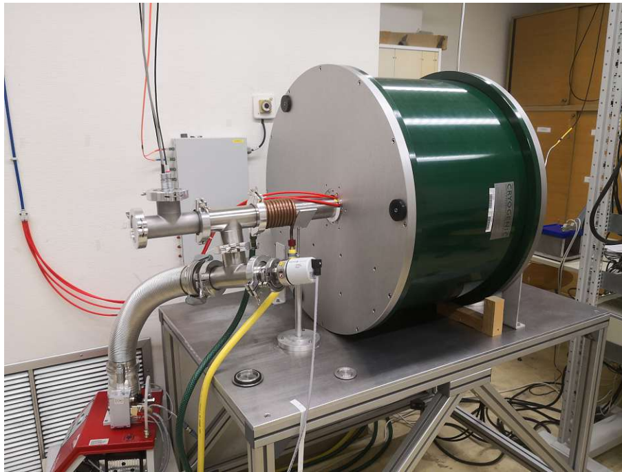
Figure 8: Magnet and vacuum pump setup with inserted sample holder. The cylindrical space inside the coil is filled with an externally water- and air cooled tube system that can be evacuated up to 10^{-6} mbar.
