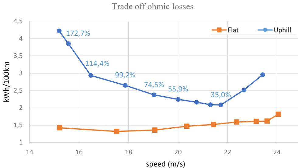
Figure 26: Ohmic losses on an uphill and flat route
