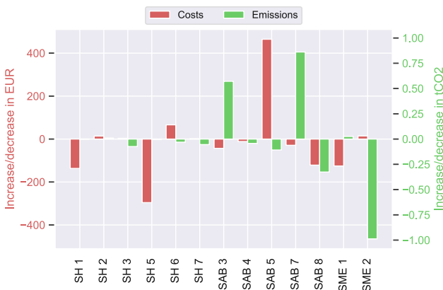
Fig. 5 Difference of annual costs and emissions between original community and new community at n = 1 (red – annual costs; green – annual emissions); increase of costs and emissions counted positive, decrease negative
