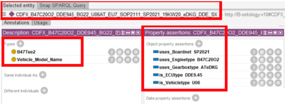
Figure 4. An instance of the class Vehicle-Model with its properties.
