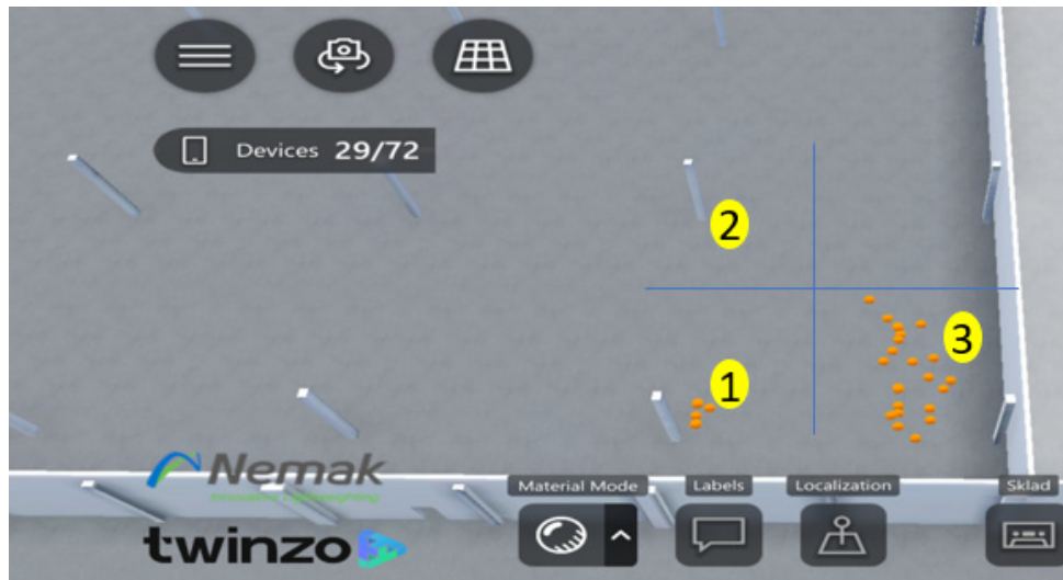
Figure 17 - 1 Active plastic tag / 2 Passive self-adhesive label / 3 Passive smart label
