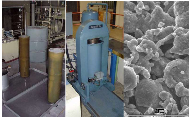
Figure 24: CIP technology and CIP microstructure (right) (own picture)
