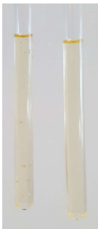
Figure A3. \text{CDCl}_3 solution of HMF before (left) and after purification (right).
