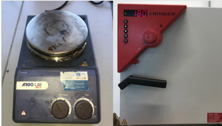
Figure 9: Devices used to heat the bitumen: Heating plate (left) and oven (right)
