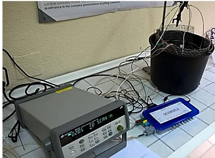
Figure 2. Practical setup for the electrochemical cell for corrosion tests.
