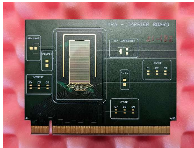
Figure 5.4: MPA2 mounted on carrier board with wire-bondings. The MPA2 pins are exposed to a PCI-E connector.
