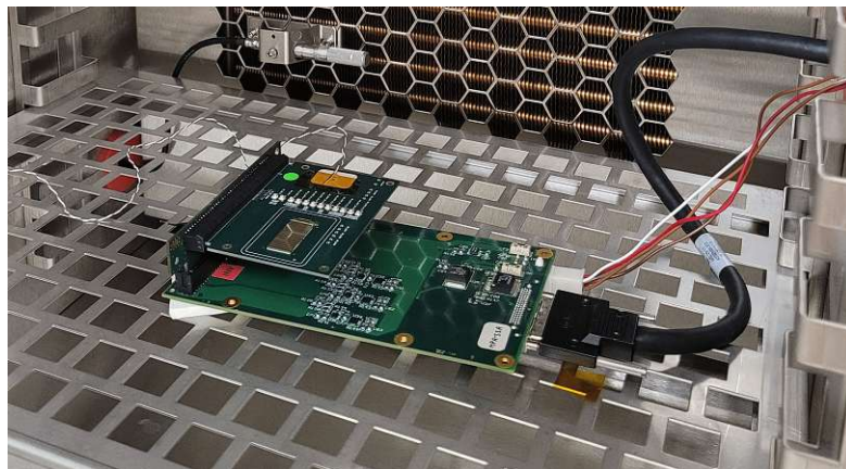
Figure 6.17: MPA2 carrier board and interface board within the ESE Climats EXCAL 1423-HA climatic chamber.
