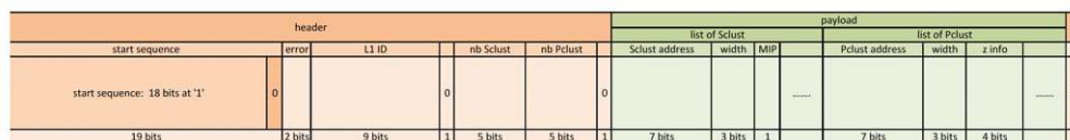
Figure 4.8: Header and payload structure of the L1 data packet [28].
