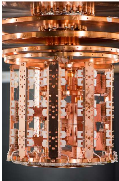
Figure 5.8.: Photo of the detector carousel of CRESST-III Run34. In this finalized state, the outer copper rails with the white plastic connectors only allow a narrow glimpse on the detectors mounted inside.
