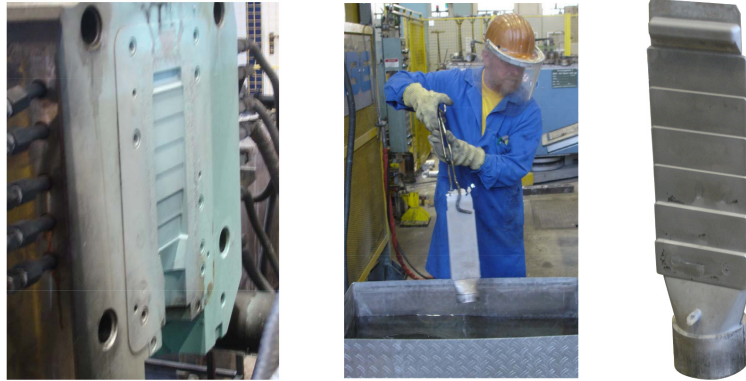
Figure 2.5: Die casting mold (left), quenching of step-bar sample (middle), step-bar sample (right); pictures courtesy of Leichtmetallkompetenzzentrum Ranshofen.
