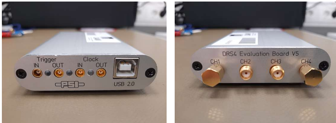
(a) The front plane of the DRS4 evaluation board. It provides the USB port for power supply as well as data transfer, trigger in-/outputs and clock in-outputs.
