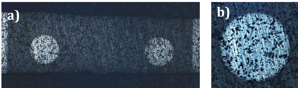
Figure 3-3: Pt-electrodes produced by sputter deposition: (a) overview of sputtered electrodes on a LLTO substrate, and (b) detail of an electrode
