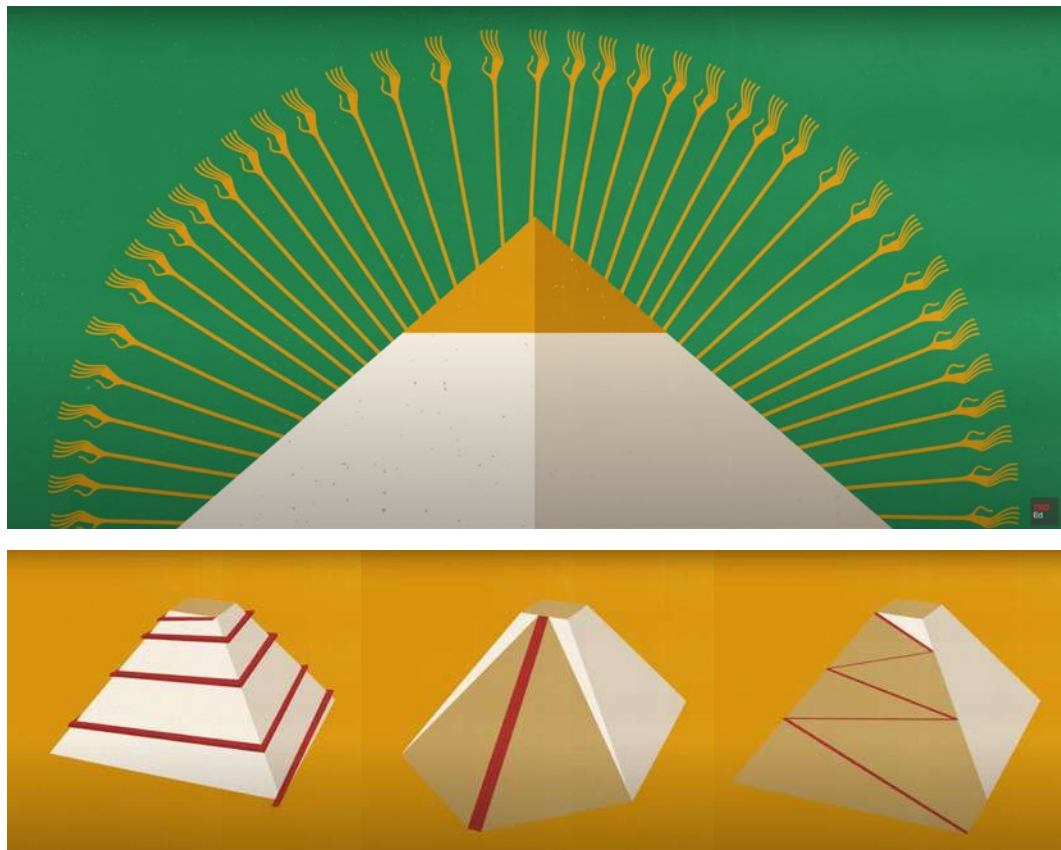
Fig. 7. Visualization of the three hypotheses of the construction of the ramp, TED-Ed, Soraya Field Fiorio
