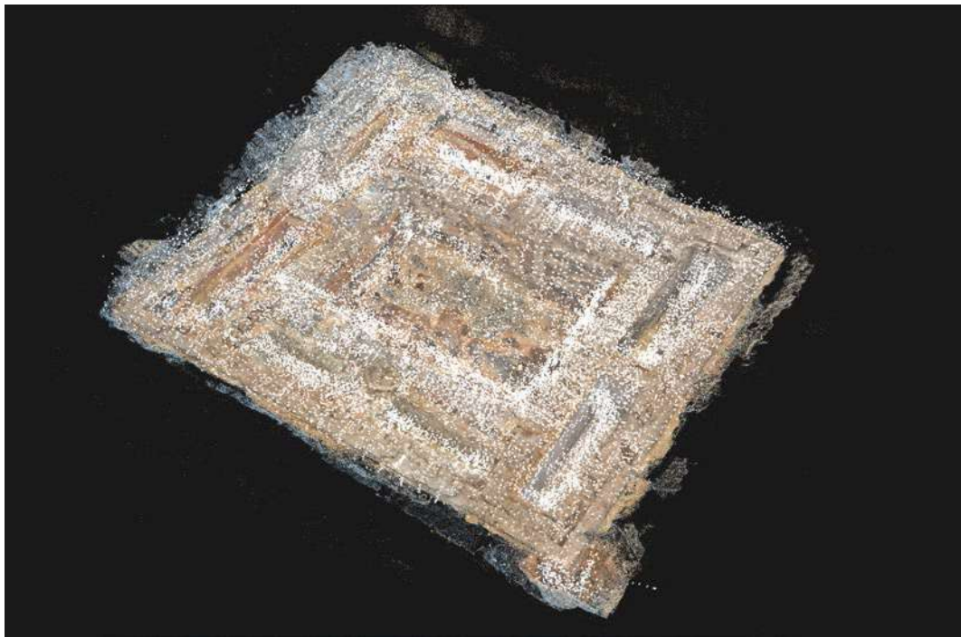
Fig. 109. Point cloud of the whole tomb with the shot photo displayed as white pyramids
