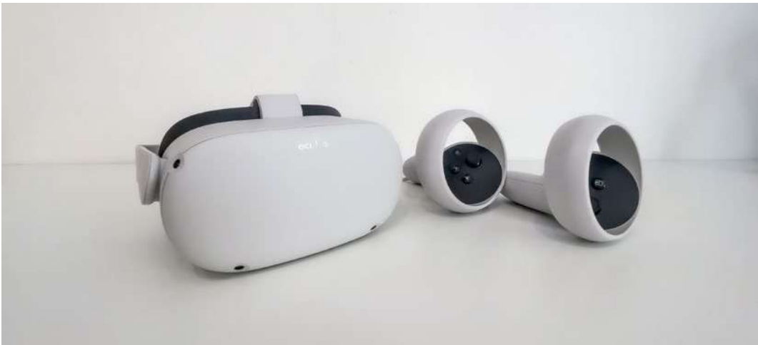
Fig. 136. Oculus Quest 2, Head mounted display and controllers
