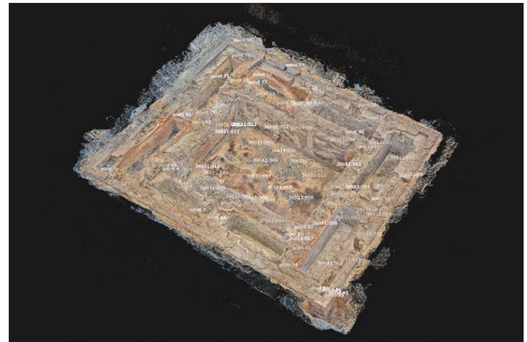
Fig. 108. Point cloud of the whole tomb with markers recognized as control points
