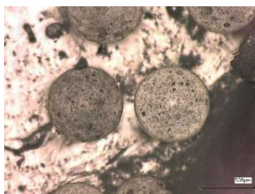
Figure 3.6: Single PS particles for depth profile analysis on a microscope slide
