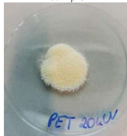
Figure 4.11: 20 h UV irradiated PET sample
