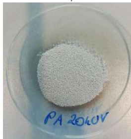
Figure 4.10: 20 h UV irradiated PA sample
