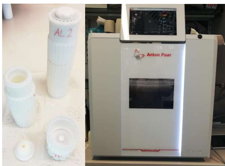
Figure 3.2: Microwave Multiwave 5000 for microwave assisted digestion Anton Paar and teflon vials as digestion vessels
