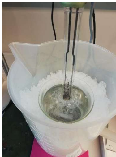
Figure 3.1: Setup artificial ageing procedure of polymer samples with dipped in UV Lamp in an ice bath cooled beaker
