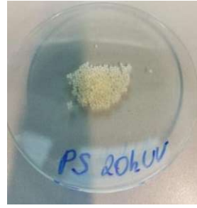
Figure 4.4: 20 h UV irradiated PS sample
