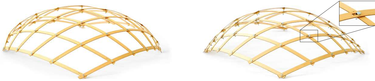
Fig. 1.3: Comparison of an elastic geodesic grid without notches (left) and with notches (right), where the target surface is a patch of a sphere. While the grid with notches shows even curvature, the grid without notches exhibits inappropriate accumulations of curvature.
