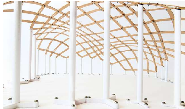
Fig. 4.2: A closeup photograph of an elastic geodesic grid dome which is also doubly-curved, fixed to 3d printed anchors. Please refer to Figure 4.20 for more examples.
