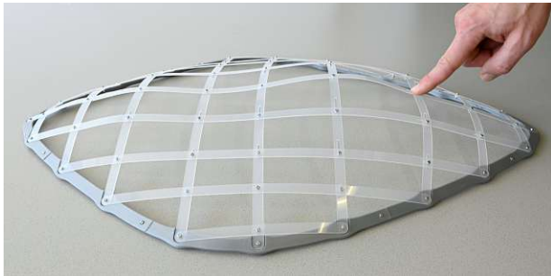
Fig. 4.1: Result of the generalized elastic grid method. An approximation of a doubly-curved surface with elliptic and hyperbolic regions using an elastic geodesic grid, deployed from a perfectly planar state by fixing its boundary elements to an anchor-ring.
