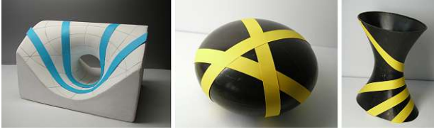
Fig. 4.5: Examples of paper strips “glued” to the surfaces. The centerlines of the strips follow geodesic curves on each surface. A sufficiently small strip can follow any geodesic on a surface but only a subset of all possible geodesics on a surface are suitable for elastic geodesic grids.
