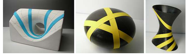
Fig. 1.8: Examples of paper strips “glued” to the surfaces. The centerlines of the strips follow geodesic curves on each surface. A sufficiently small strip can follow any geodesic with non-vanishing curvature. Adapted from [Pottmann et al. 2015].
