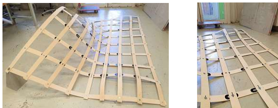
Fig. 3.15: One module of the failed medium-scale model. The structure is not able to carry its self-weight. Some curvature features can be recognized, however, the structure as a whole performs rather poorly.
