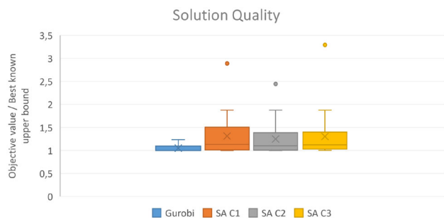
Fig. 15 Box plots comparing the overall results achieved on the set R_6 . The vertical axis measures the achieved relative objective values (solution cost produced by each method divided by the overall best found solution cost) (Color figure online)
