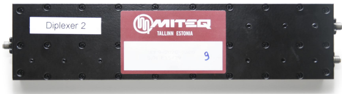
Figure 5.8: The duplex filters used in the S-band RF front end to separate the receive and the transmit frequency bands.
