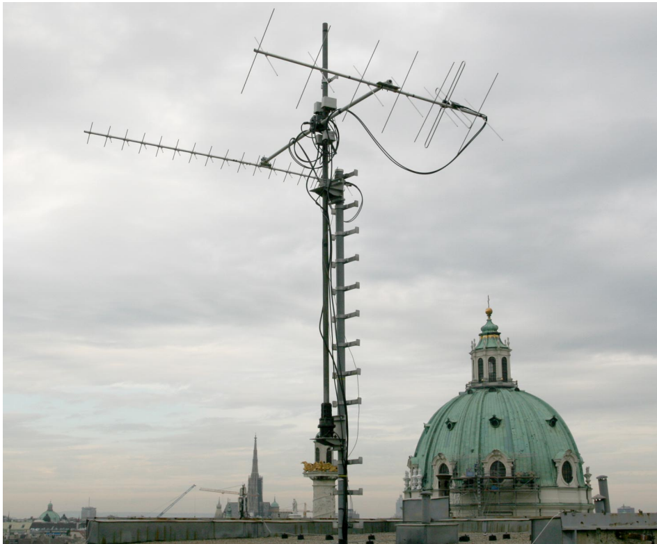
Figure 5.31: Photo of an early test setup of one VHF and one UHF Cross-Yagi antenna completed with LNA and polarization selector mounted on a second azimuth/elevation rotator.
