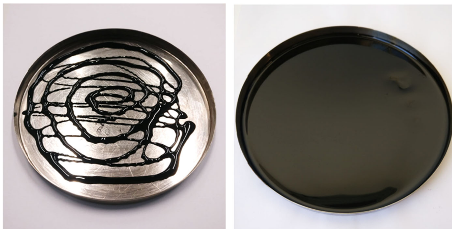
Fig. 1 Bitumen in metal container before (left) and after (right) PreVBA
