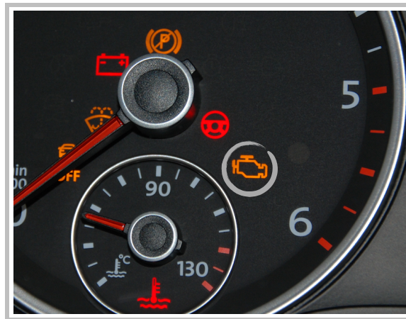
Figure 5.1: The Malfunction Indicator Lamp (MIL) on the dashboard of a VW Tiguan
