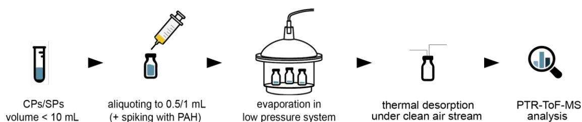
Figure 13. Schematic step-by-step approach of the sample preparation method used for cloud water samples. A more detailed description of the used setup is given in Materić et al. (2017) (Materić et al. 2017).
