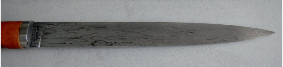
Figure 7: Knife blade forged from the Campo del Cielo meteorite.
