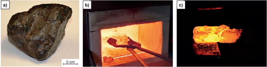
Figures 1a to c: Forging a Campo del Cielo meteorite. a) Meteorite in its initial state, b) red-hot meteorite in the electric furnace, c) meteorite during the forging process. It can already be recognized that the meteorite starts to break apart.
