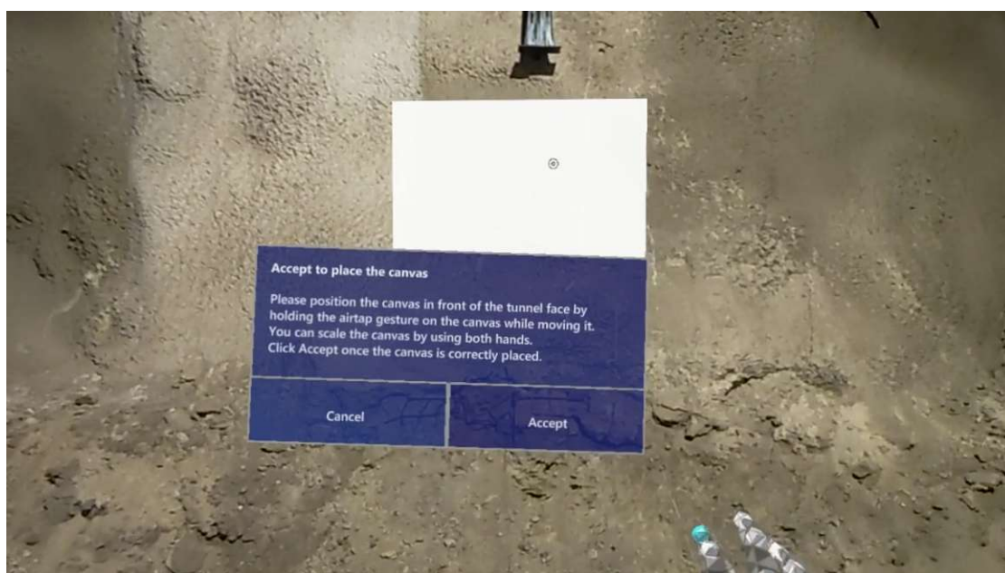
Figure 7.21: The canvas placed for the tunnel face mapping.
