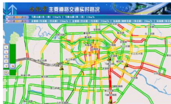
Figure 4.2: Example for colour encoding to visualise congestion in a road map of Hefei [79].
