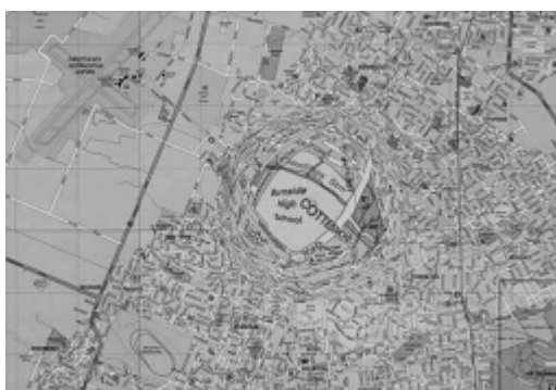
Figure 3.10: Example of a focus + context interface using the fisheye technique to show detailed information of a focused region within surrounding context [18].
