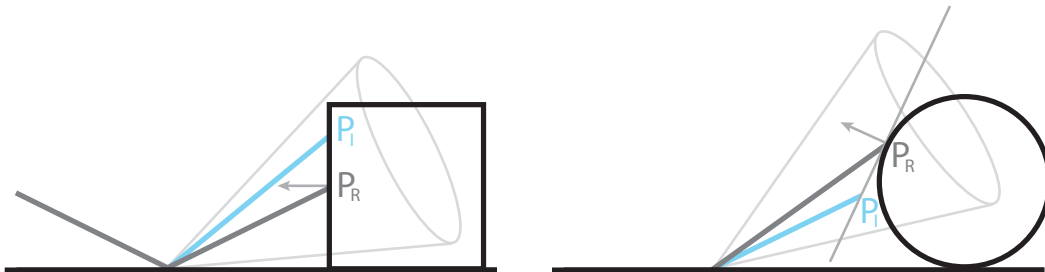
Figure 4.29: The world position P_R and the surface normal of the reflected scene geometry are known at the perfect reflection direction \omega_r (dark gray). The scene is then locally approximated by the tangent plane of P_R to obtain approximative positions P_I where other sampling rays (blue) within the lobe intersect the scene. This assumption is correct for planar reflected surfaces, for arbitrary surfaces the error depends on local scene curvature and specular lobe width.
