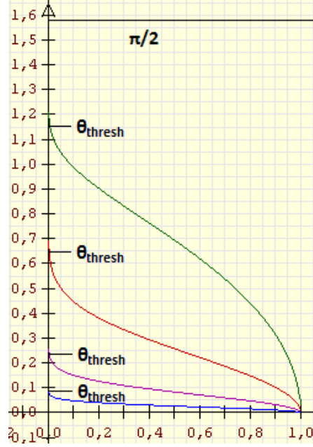
Figure 4.13: This plot shows how numbers \xi_1 \in (0, 1] (on the x-axis) are transformed to half-angles \theta_h \in (0, \pi/2] (on the y-axis) when using the non-linear importance transformation function in Eq. 4.6 for different lobe parameters (different colors). At \xi_1 = 0 , the resulting \theta_h is \pi/2 , which ensures that no directions are excluded for unbiased integration, but in fact, the portion with significant importance ends before \xi_1 reaches 0. Identifying the \theta_{thresh} -angle for a particular \xi_1 -value close to zero, where the slope of the transformation curve starts to get very steep, yields an estimate of the lobe extent worth sampling.
